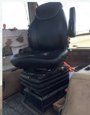
Air LGV90/CIAR TT fitted to John Deere 8400 tractor
